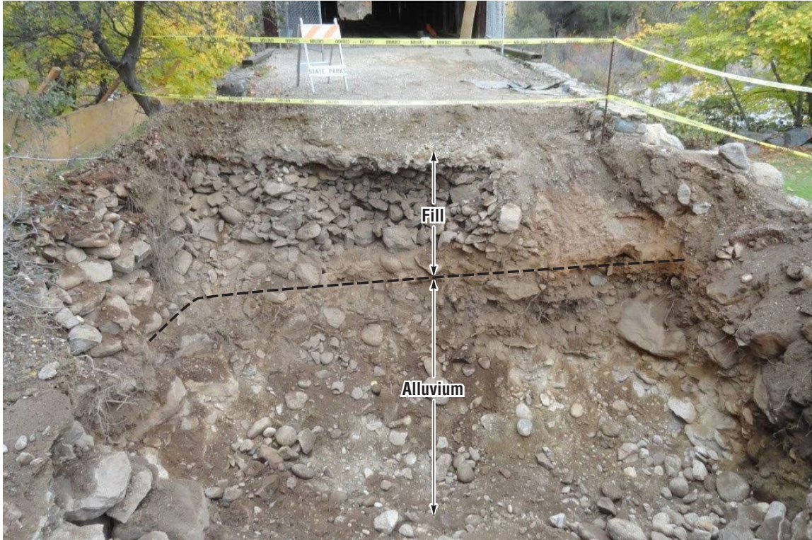
Photo No. 7 Typical subsurface conditions – south abutment area
