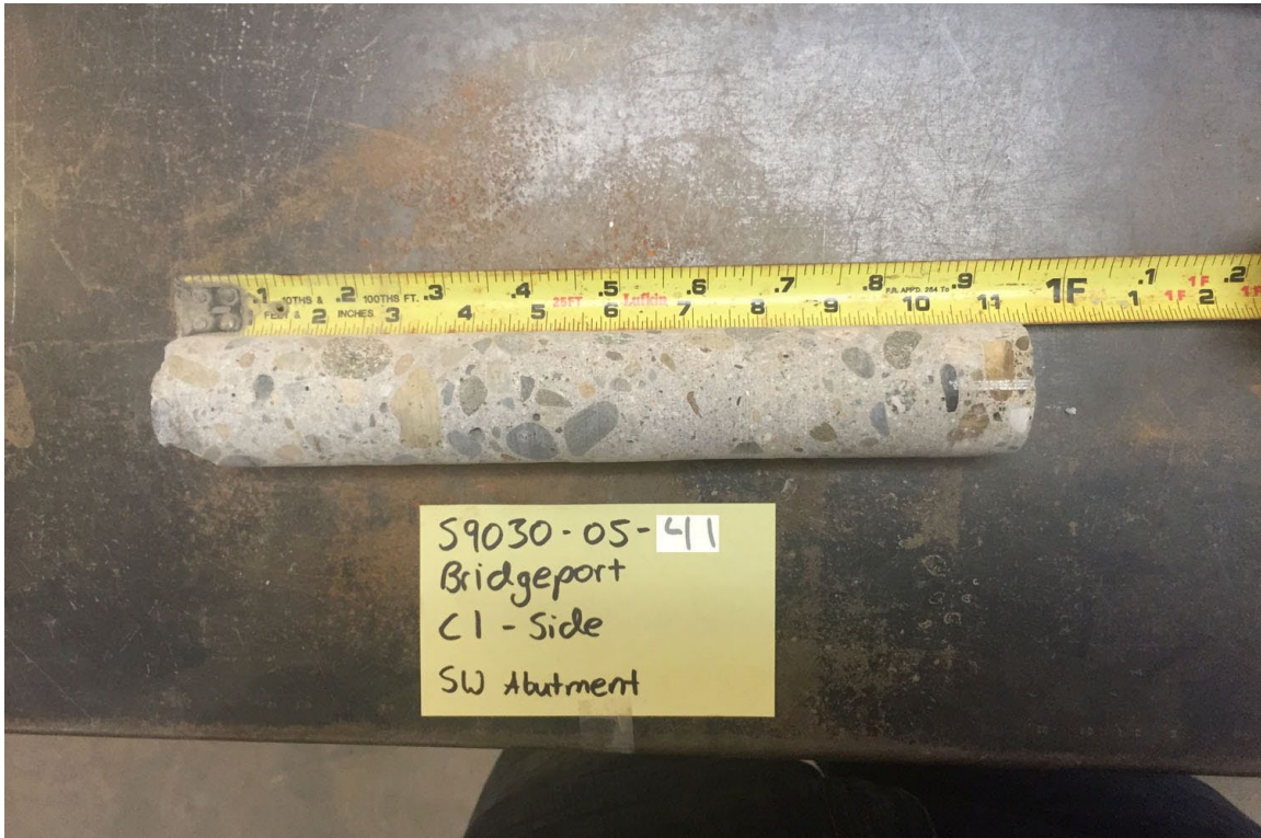
Photo C1 Core C1 – south abutment arch seat
